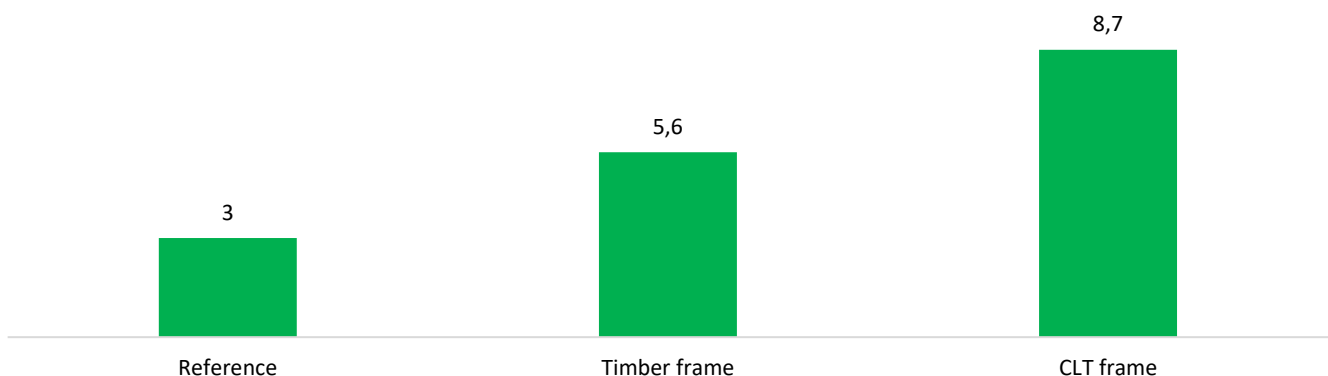
Impact of the wood structure scenarios to the carbon handprint (average of residential, office and school buildings)
